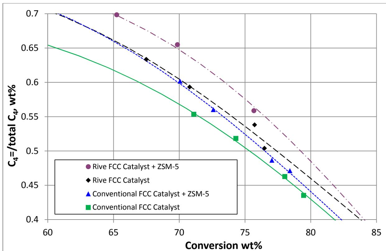
**Figure 12: Higher C<sub>4</sub> Olefinicity for Optimized Rive Catalysts with ZSM-5 Additive**
