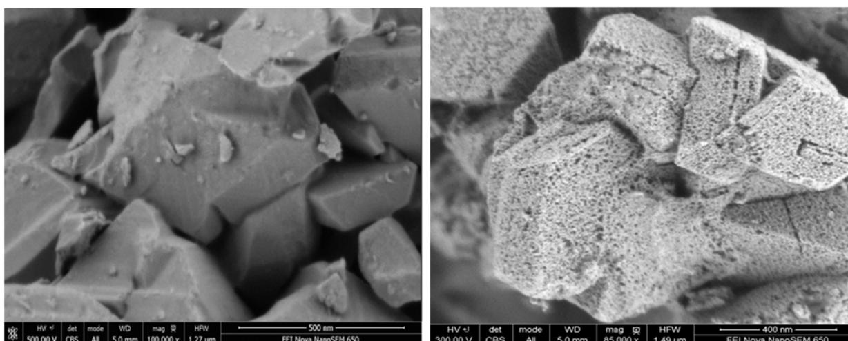
**Figure 1: Photomicrographs of Conventional Zeolite (left) and Rive Zeolite (right)**
