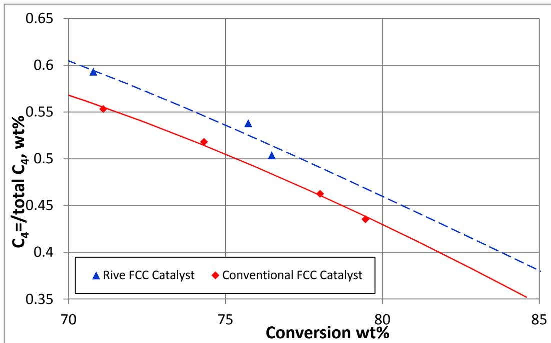
**Figure 5: C<sub>4</sub> Olefinicity for Optimized Rive Catalyst Formulation**
