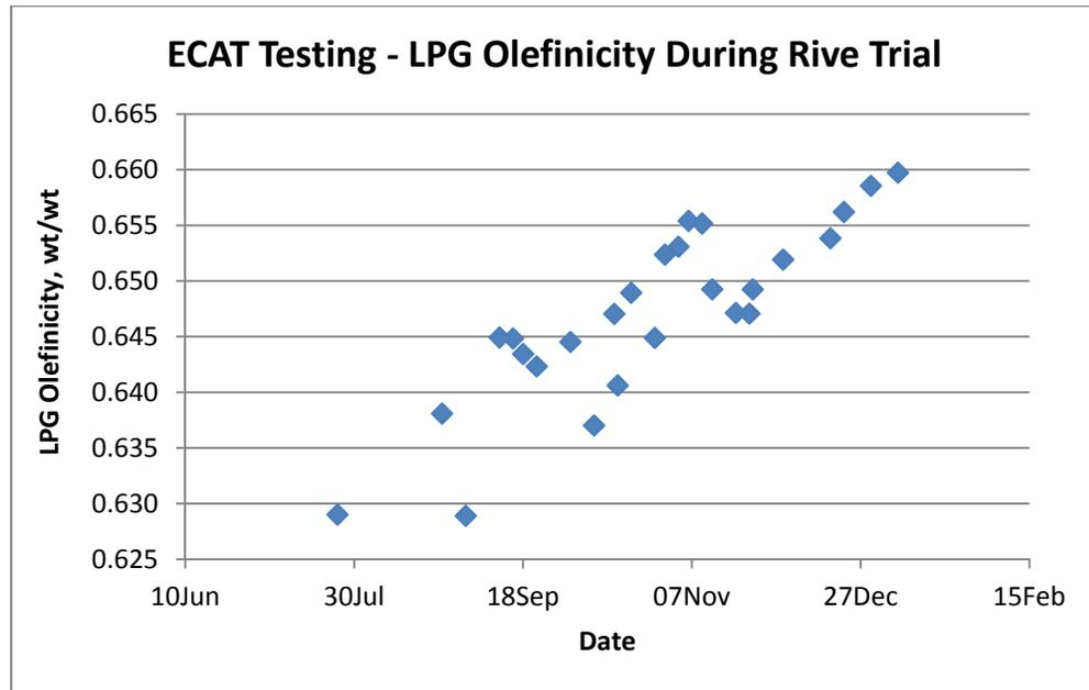
Figure 6: ACE Testing of ECAT Shows Higher LPG Olefinicity with Rive
