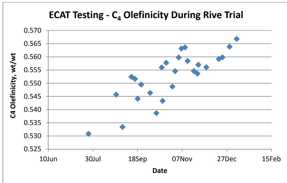
Figure 7: ACE Testing of ECAT Shows Higher C<sub>4</sub> Olefinicity with Rive
