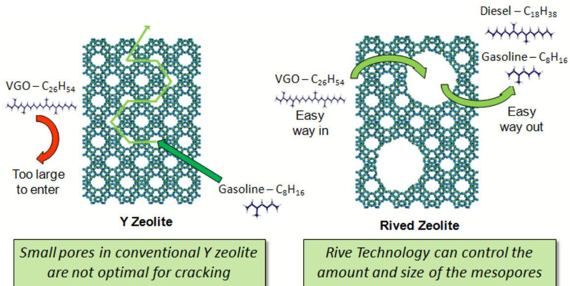
**Figure 3: Overview of Rive's Molecular Highway™ Technology**
