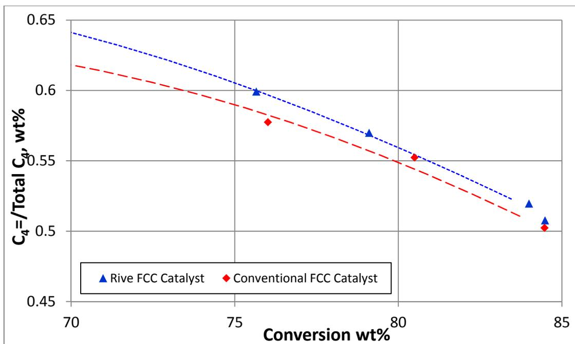
**Figure 4: Rive's Effect on C<sub>4</sub> Olefinicity**
