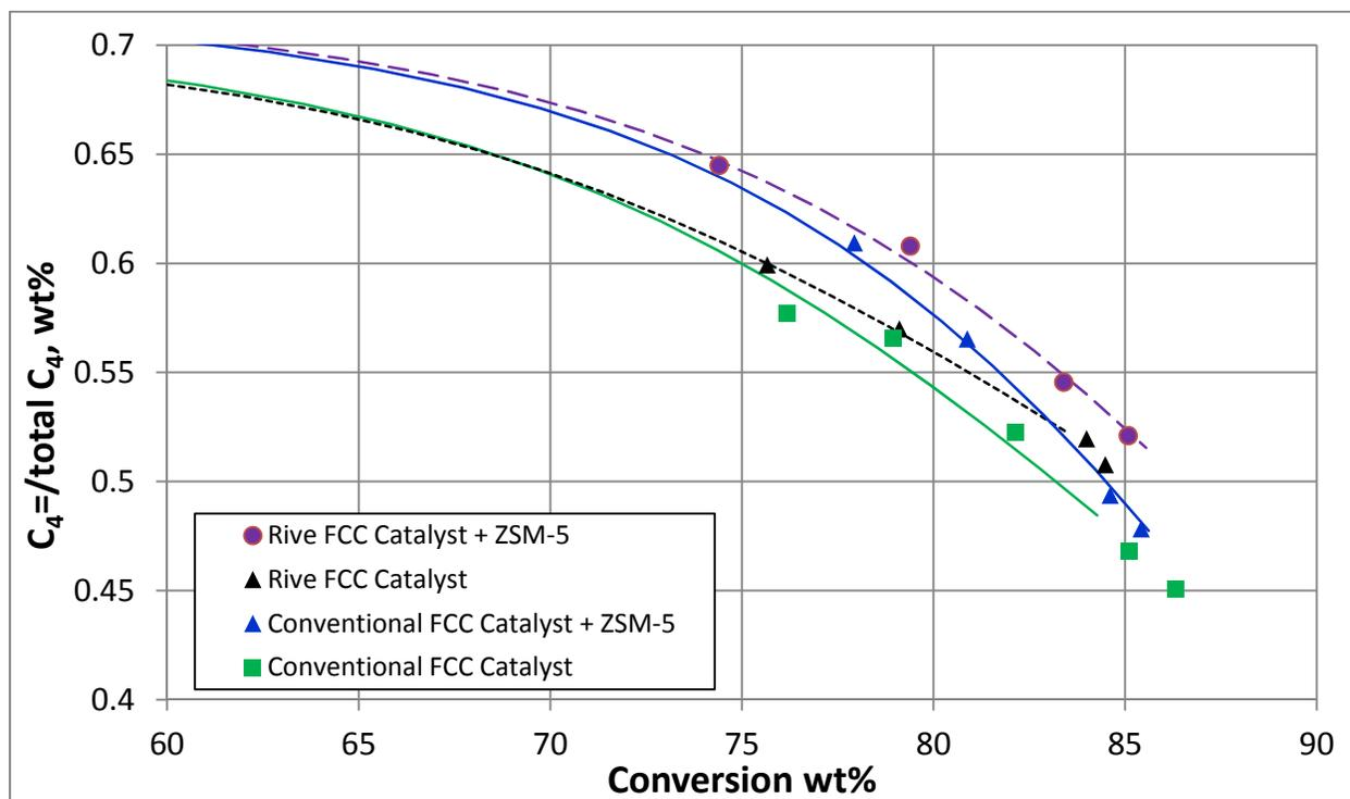
**Figure 11: Higher C<sub>4</sub> Olefinicity for Rive Catalysts with ZSM-5 Additive**
